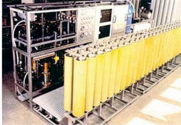
From a cost and convenience perspective, it is best to have a high packing density because the greater the density, the greater the membrane area enclosed, the lower the cost of the membrane element. The downside of high density membrane elements is the greater likelihood of fouling.
